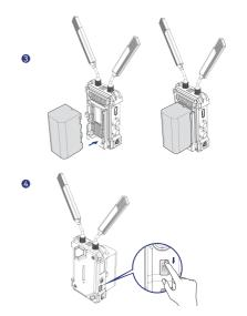
3. Install the battery (Support NP-F batteries or DC power adapter) 4. Toggle the power switch downward to turn on the transmitter.
